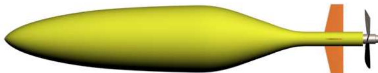
Figure 2.5: Laminar form hull
